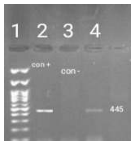
Figure 3: Agarose gel electrophoresis of the S. uberis PCR products. Lane 1: 100 bp DNA marker; lane 2: positive control (445 bp); lane 3: negative control and lane 4 is a positive sample.
