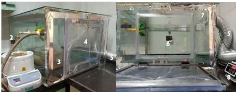
Figure 1: The vivarium that designed to expose laboratory animals to petroleum vapors. Different parts are marked with numbers, 1) heater with timer, set specified temperature 2) erlen to evaporate crude oil 3) rat cage 4) Entrance door of vivarium chamber 5) Tube for removing of pollutants 6) thermometer 7) Pollutant output fan 8) Output fan timer
